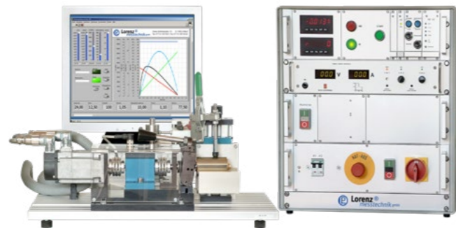
DC-Low-Voltage Motor Test Bench:
